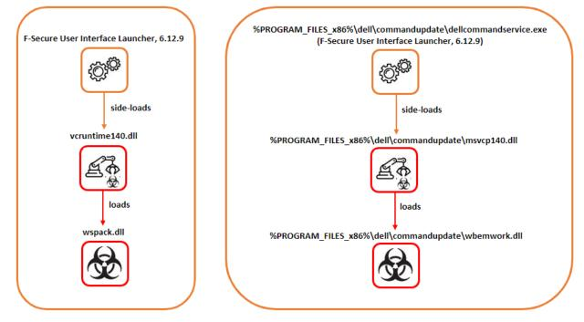
F-Secure has been informed of the binary abuse to perform side-loading of malicious DLLs used in the attack. F-Secure acknowledged that, as the binary was used independently, outside of the normal software functionality, no further action is required. The F-Secure product installed on a system is not vulnerable to the DLL side-loading abuse.
