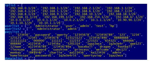
Fig 2. Hardcoded usernames, passwords and subnets to scan
