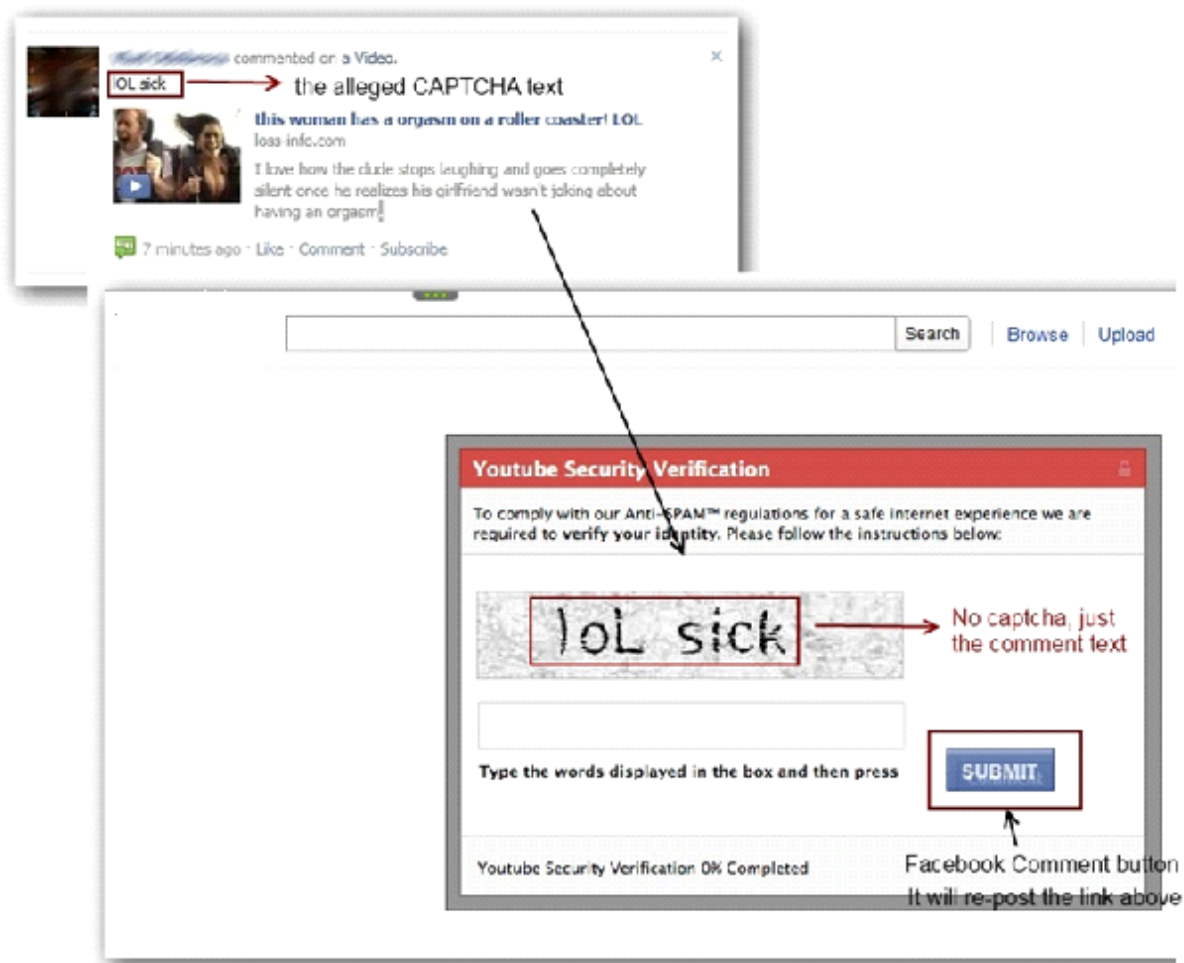
Figure 8: Propagation mechanism of a Facebook worm. The CAPTCHA is actually the comment
